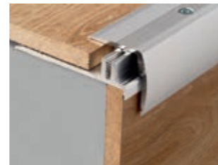
5 Stair nose, aluminium PGSTPSILVME250, 2500 x 30 x 25 mm Fits flooring thickness of 7 - 15 mm. Surface: aluminium. Colour: silver.
